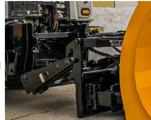
Detail view of the LPM 500 hitch connecting to the hitch plate.
