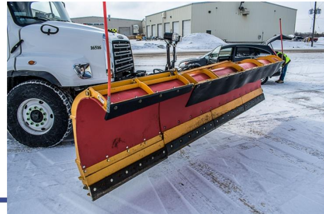
Extension fully deployed for seamless moldboard
