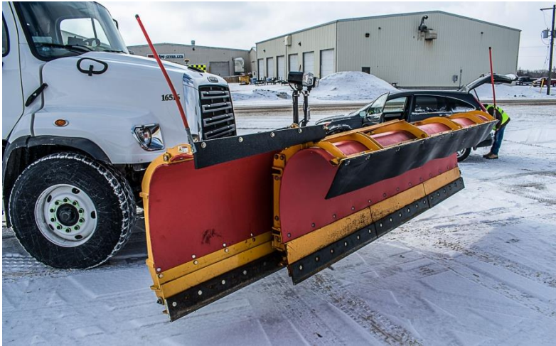
Plow with partially deployed extension
